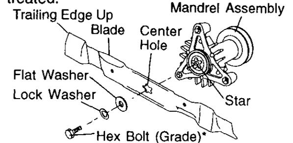
\*A Grade 8 heat treated bolt can be identified by six lines on the bolt head.
