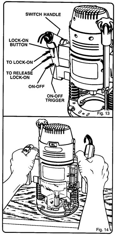
The proper rate of feed depends on several factors: the hardness and moisture content of the wood, the depth of cut, and the cutting diameter of the bit. When cutting shallow grooves in soft woods such as pine, a faster rate of feed can be used. When making deep cuts in hardwoods such as oak, a slower rate of feed will be required.
