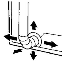
4. Use the straightest path possible when routing the exhaust vent. Use the fewest number of elbows and turns. Allow room when using elbows or making turns. Bend vent gradually to avoid kinking.
