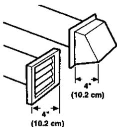
3. The exhaust vent can be routed up, down, left, right, or straight out the back of the dryer. Space requirements are listed in your Installation Instructions.
