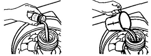
Dilute liquid fabric softener by filling the dispenser with warm water until liquid reaches the crossbar in the opening.
