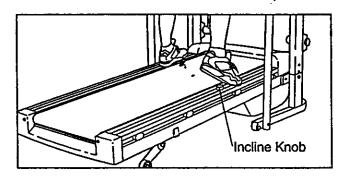
To decrease the incline, stand with your left foot towards the front of the left foot rail. Using your right foot, press down the foot incline knob until the desired incline is reached. Note: It may be helpful to step off the treadmill when pressing down on the incline knob to decrease the incline.
