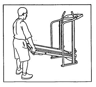
2. Move your right hand to the position shown and hold the treadmill firmly. Raise the treadmill until the storage latch closes over the frame guide. Make sure that the storage latch closes fully over the frame guide.
