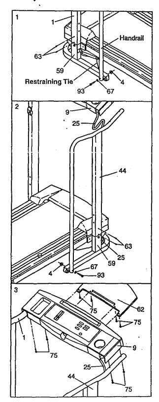
4. With the help of a second person, carefully lower the Left and Right Uprights (1, 44) until the handrails are resting on the floor.
