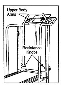
To vary the intensity of your upper body exercise, the resistance of the upper body arms can be adjusted. To increase the resistance, turn the resistance knobs clockwise; to decrease the resistance, turn the knobs counterclockwise.
