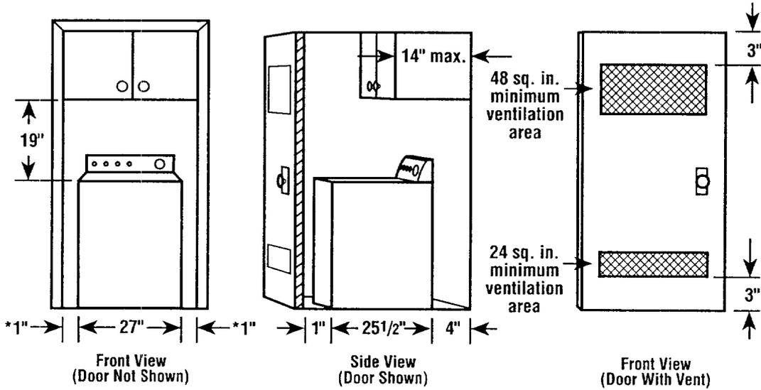
\*Additional clearance for wall, door and floor moldings may be required.
