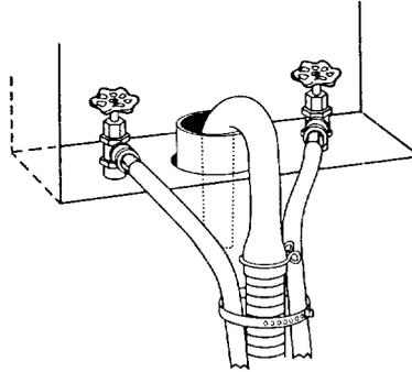
**STEP 2.** Locate the remaining piece of shipping strap (not the end with the three cotter pins) from STEP 4 of "REMOVE SHIPPING STRAP." Use it to wrap the drain hose together with the laundry tub or standpipe. Push fastener into the nearest hole in the shipping strap.
