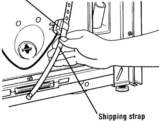
**STEP 4.** Cut the shipping strap about 16 inches from plug end. Look for the words "CUT HERE." Discard end with three cotter pins. Slide remainder of shipping strap from the electrical plug. You will use this to secure the drain hose.
