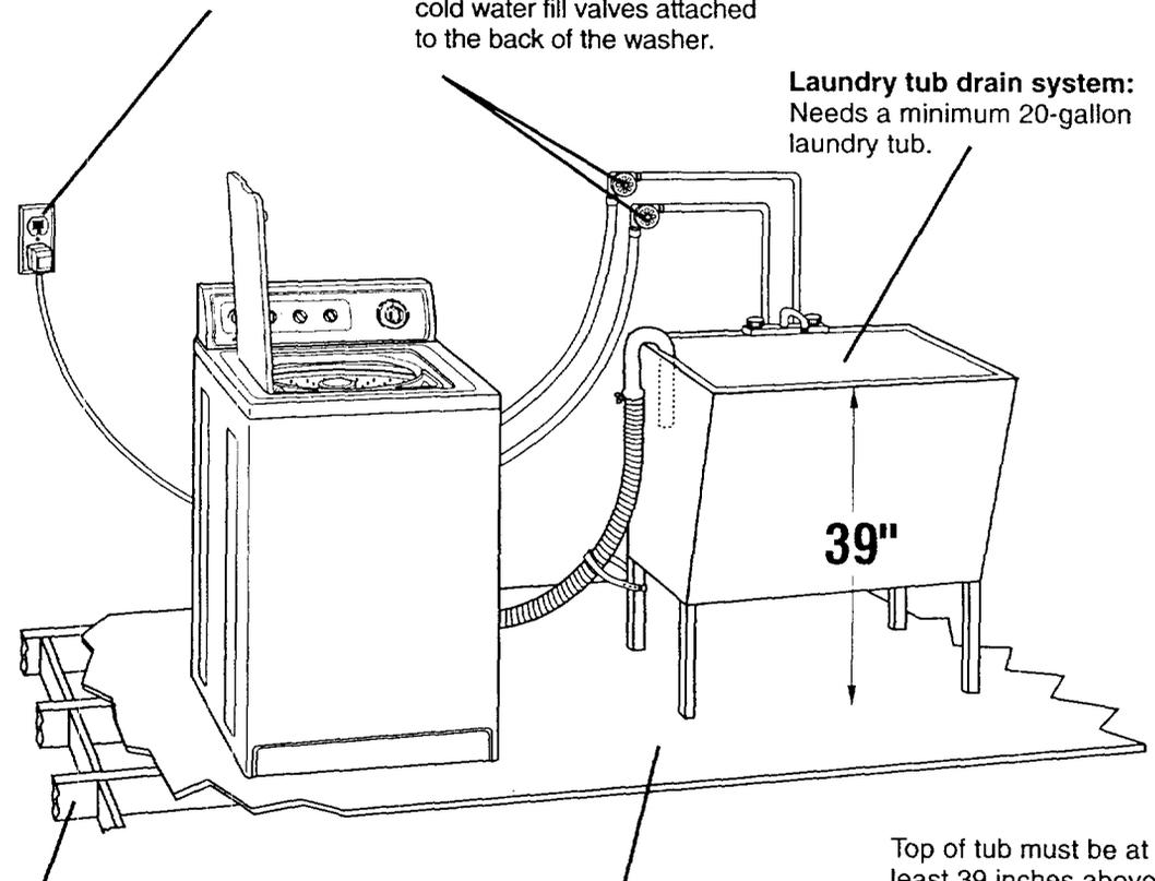
**Support:** Floor must be sturdy enough to support a total weight of 315 pounds (including washer, water, and load weight).
