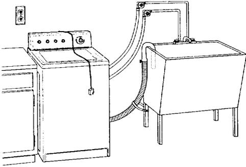
If the water faucets and drain standpipe are recessed, put hooked end of drain hose in standpipe. Tightly wrap the shipping strap around the drain hose and water inlet hoses (not the handles or stems). Push fastener into the nearest hole in the shipping strap.
