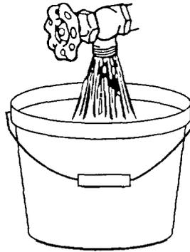
**STEP 2.** Attach the hose with the red coupling to the hot water faucet. Screw on coupling by hand. Make an additional two-thirds turn with pliers to tighten coupling. **DO NOT OVERTIGHTEN;** this could damage the coupling.
