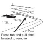
To replace or relocate: Line the shelf up with the supports and slide it into place. The shelf can be repositioned when the door is at 90° or more. To reposition the shelf, slide the shelf past the stops
