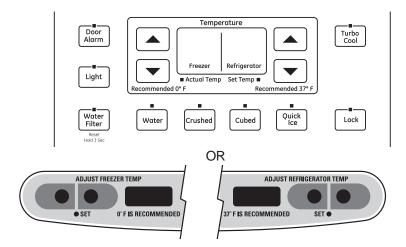
The temperature controls are preset in the factory at 37°F (2.8°C) for the refrigerator compartment and 0°F (-17.8°C) for the freezer compartment. Allow 24 hours for the temperature to stabilize to the preset recommended settings.
