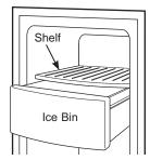
To reach the power switch, pull the shelf straight out. Always be sure to replace the shelf.
