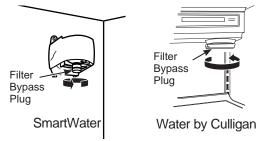
To use the filter bypass plug on Water by Culligan<sup>™</sup> models, you must first remove the filter adapter from the cartridge holder by turning it to the left.
