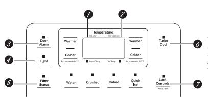
The temperature controls are preset in the factory at **37°F (2.8°C)** for the refrigerator compartment and **0°F (-17.8°C)** for the freezer compartment. Allow 24 hours for the temperature to stabilize to the preset recommended settings.
