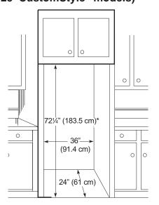
\*72-1/4" (183.5 cm) required for full adjustment of mobility wheels. If cabinets installed above refrigerator have doors that are flush to the top of the opening for the refrigerator, then an additional 1/8" may be required to provide clearance for cabinet doors to open freely.
