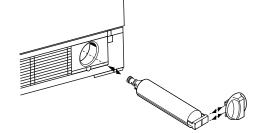
**3.** Take the new water filter out of its packaging and remove the cover from the O-rings.
