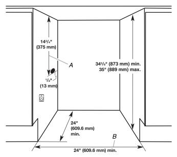
Critical Dimensions: A. Utility opening B. Minimum opening width
