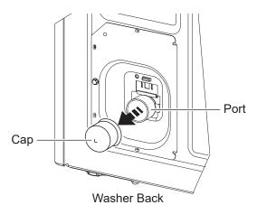
Connect drain hose to drain port on back of washer. Open clamp with pliers and slide onto hose end. Holding clamp open, push hose end onto drain port until fully seated. Release clamp between locating ribs on hose end. Outlet of hose end should be oriented vertically.
