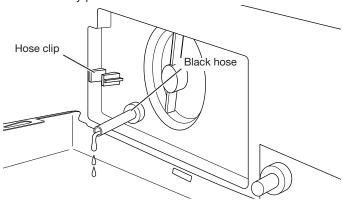
3. Lay a cotton cloth beneath the drain pump filter to absorb any water still in it. Then remove the drain pump filter by turning it counterclockwise.
