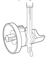
5. Reinsert the drain pump filter by turning it clockwise. Make sure to turn it in as far as it will go, with the filter handle remaining as close as possible to the vertical position.
