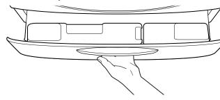
Open the dispenser drawer by pulling on the handle at the base of the washer. If desired, the drawer can be completely removed from the washer.
