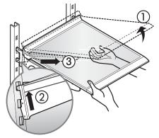
**To reinstall a shelf:** With front of shelf angled slightly up, engage hooks on back of shelf into attachment slots, and then lower front of shelf into place.
