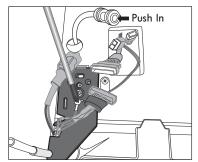
**3.** Using a large phillips screwdriver, turn top hinge fastener counterclockwise to remove the top hinge plate.
