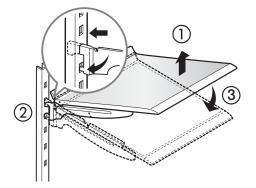
**CAUTION:** Make sure that shelves are level from one side to the other. Failure to do so may result in the shelf falling or spilling food.
