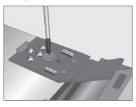
**3.** Lift the door from the middle hinge pin and remove the door. Place the door, inside facing up, on a non-scratch surface.
