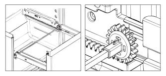
2. Fully push in and close freezer drawer to engage rails with rail support locking tab, applying a bit of pressure after the door is closed to seat the tabs to the rail.
