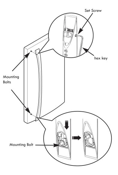
**NOTE:** Removing the doors is always recommended when it is necessary to move the refrigerator through a narrow opening. If it is necessary to remove the handles, follow the directions below.
