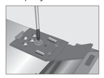
3. Screw top hinge cover into place with a screwdriver.
