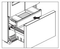
5. Open and close the freezer drawer several times to make sure operation is smooth and seal is consistent all the way around the freezer compartment.
