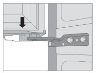
**2.** Fit the top hinge over the mounting holes and align to proper position before tightening.
