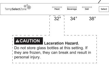
**Note:** Temperatures indicate the appropriate temperatures for the food and actual temperatures may vary based on normal operation and other factors such as door openings and fresh food set point.
