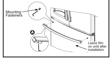
Reinstall the handles using the same procedure as removing.
