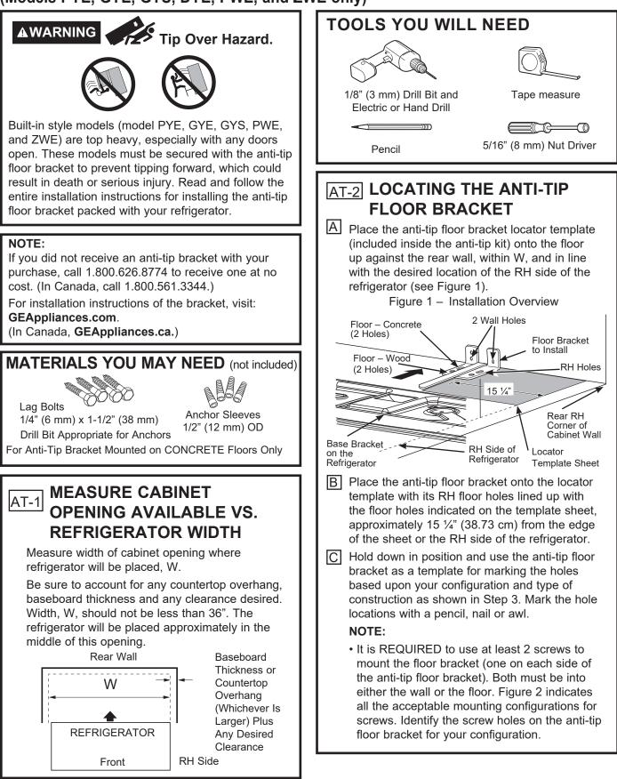
**INSTALLING THE REFRIGERATOR (Cont.)** Anti-Tip Floor Bracket Installation (Models PYE, GYE, GYS, DYE, PWE, and ZWE only)
