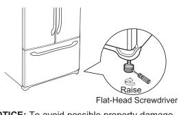
**NOTICE:** To avoid possible property damage, the leveling legs must be firmly touching the floor.
