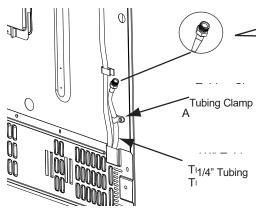
If you are using the SmartConnect<sup>™</sup> tubing, the nuts are already assembled to the tubing.
