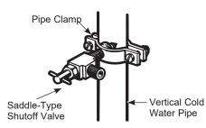
**NOTE:** Commonwealth of Massachusetts Plumbing Codes 248CMR shall be adhered to. Saddle valves are illegal and use is not permitted in Massachusetts. Consult with your licensed plumber.
