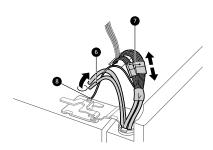
3 Rotate the hinge lever **9** counterclockwise. Lift the top hinge @ free of the hinge lever latch 🛈.
