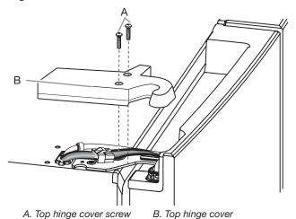
2. Disconnect the water dispenser tubing located on top of the door hinge. Firmly pull up on the clasp. Then, pull the tubing out of the fitting.
