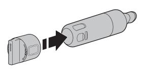
6. Insert the filter into the housing.
