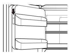
Turn on the ice maker by moving the switch to the On (I) position.
