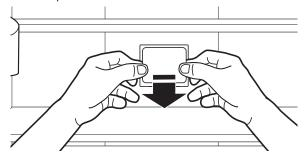
**NOTE:** When cover is removed for the first time, a small foam part the size of the filter will need to be discarded.
