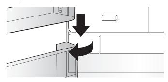
2. Twist the water filter and turn 90° counterclockwise to unlock.
