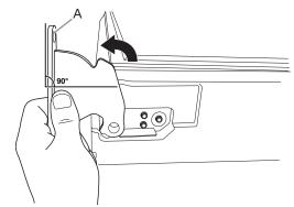
A. Hinge base turned to a  $90^{\circ}$  angle with the bottom edge of the door
