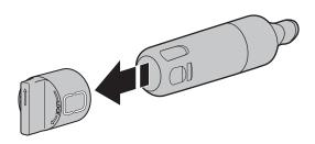
5. Install the water filter cap onto the new filter. Be sure to align the arrows so the groves in filter align with ribs in filter cap.
