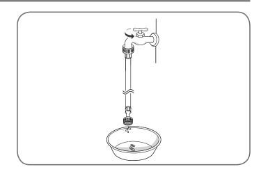
3. Always run a gallon or two of water through each inlet hose to flush dirt, scale and other debris out of the water lines. Doing so will help prevent future problems with clogged filter screens, and will also allow you to verify which hose is hot and which is cold.
