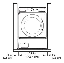
Allow at least 25 <sup>13</sup>/16 in. (65.5 cm) in front of the washer to open the door.
