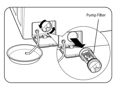
Twist the pump filter counterclockwise to remove. Remove any lint and foreign objects from the pump filter. Insert pump filter back into opening and twist clockwise to secure. Be sure to close the drain pump filter access panel.
