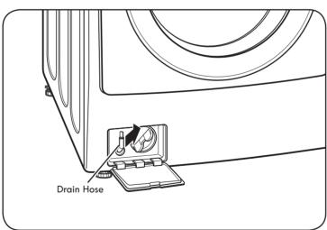
2 Unclip the drain hose and pull it out. Place the end of the drain hose into a shallow pan or a floor drain. Make sure not to pull the hose out too far, or it may not drain properly.
