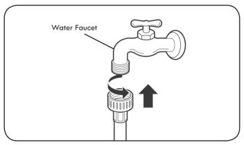
2. Connect the water supply hoses to the HOT and COLD water faucets tightly by hand and then tighten another ½ turn with pliers.
