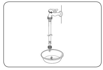
3. Always run a gallon or two (4L) of water through each inlet hose to flush dirt, scale and other debris out of the water lines. Doing so will help prevent future problems with clogged filter screens, and will also allow you to verify which hose is hot and which is cold.
