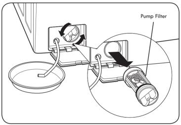
Twist the pump filter counterclockwise to remove. Remove any lint and foreign objects from the pump filter. Insert pump filter back into opening and twist clockwise to secure. Be sure to close the drain pump filter access panel.
