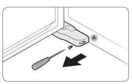
1. With the freezer door open, use a Phillips head screwdriver to remove the screw holding the cover (A) of the adjustable leg.
