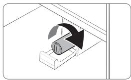
**4.** Insert a new filter cartridge. Use only Samsung-provided or approved filters.
