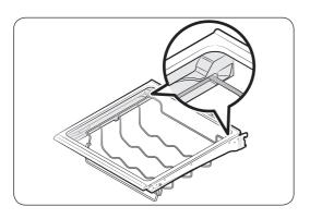
Insert the wine rack under the shelf of the fridge. Make sure to insert it all the way to the end as shown in the figure.
