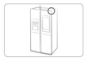
Door gaps can be corrected using the gap bolt on the top right corner of the refrigerator.
