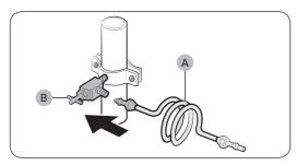
Connect the water line installation kit(A) to the shut off valve (B).
