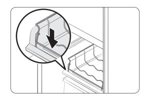
Insert the wine rack on top of the sliding shelf of the FlexZone, which is normally below the partition guide.
