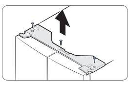
**1.** With the door closed, use a Phillips head screwdriver to remove the screws (x3) in the **top cover**. Then, carefully remove the **top cover** along with the wire connectors.
