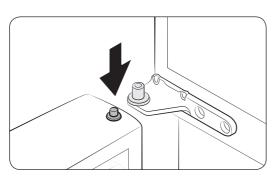
**2.** While pressing the hinge shaft down, position the door so that the hinge shaft is below the shaft hole in the middle hinge. Release the hinge shaft so that it enters the shaft hole.
