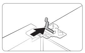
**3.** Insert the clamp in the direction of the arrow.
