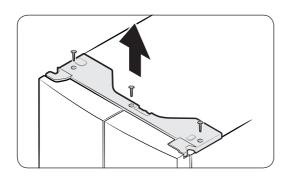
1. With the door closed, use a Phillips head screwdriver to remove the screws (x3) from the top cover. Pull up and remove the top cover with the connectors.
