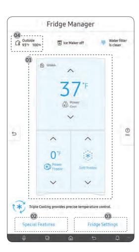
The Fridge Manager is a graphical representation of your refrigerator. The top half represents the refrigerator compartment, the bottom left the freezer compartment, and the bottom right the FlexZone. The temperature or mode settings for each are displayed over each section.
