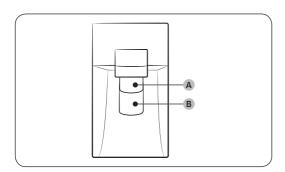
The water dispenser offers 3 options: chilled water, cubed ice, and crushed ice. If you do not want to dispense ice, simply press the water lever (B).
