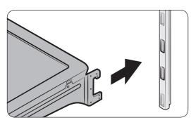
To reinsert, hold the shelf at an angle so the front is higher than the back, and then insert the top hook into the top shelf notch. Then, lower the shelf and insert the bottom shelf hook into the bottom shelf notch.
