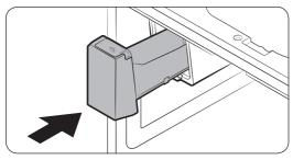
**3.** When done, put the bucket back into position. If the bucket does not fit in, turn the helix screw 90 degrees, and then try again.
