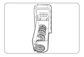
If the bucket does not fit in, turn the helix screw 90 degrees, and then try again.
