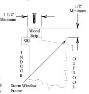
Mobile home window installation Add wood strip (at least 1 1/2" wide) along entire width of window sill. Thickness of wood strip should match height of front lip on window frame. Fasten wood strip to sill with a minimum of three countersunk wood screws (not supplied with kit). This provides a smooth surface for mounting air conditioner.
