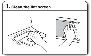
Clean the lint screen before each load. Pull the lint screen out of its holder. Roll lint off the screen with your fingers. Do not rinse or wash screen to remove lint. Push the lint screen firmly back into place.
