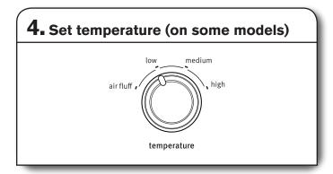
Select temperature by turning the knob to the desired position or select the Automatic Dry Cycle that has the temperature included in the cycle selections. See "Setting the Drying Temperature".
