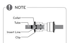
1) Gently press the Collet and insert the tube until only one line shows on the tube.
