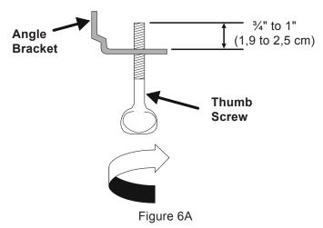
4. Once the cooktop is installed, clamp the unit down as shown (Fig. 6).
