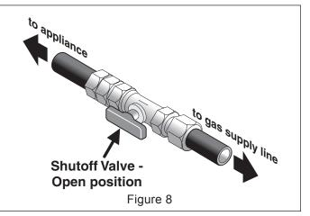
Once regulator is in place, open the shutoff valve in the gas supply line. Wait a few minutes for gas to move through the gas line.
