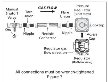
Assemble the flexible connector from the gas supply pipe to the pressure regulator in the following order: 1. manual shutoff valve
