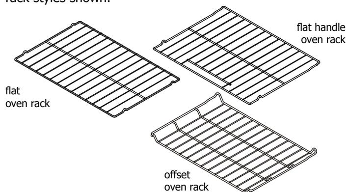
The **flat oven rack** or **flat handle oven rack** (some models) may be used for most cooking needs.
