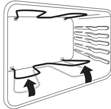
Figure 19: Lift bake element
