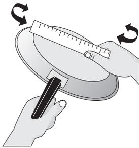
Check for flatness by rotating a ruler across the bottom of the cookware (see Figure 1). Cookware should have flat bottoms that make good contact with the entire surface heating element (see Figure 2).
