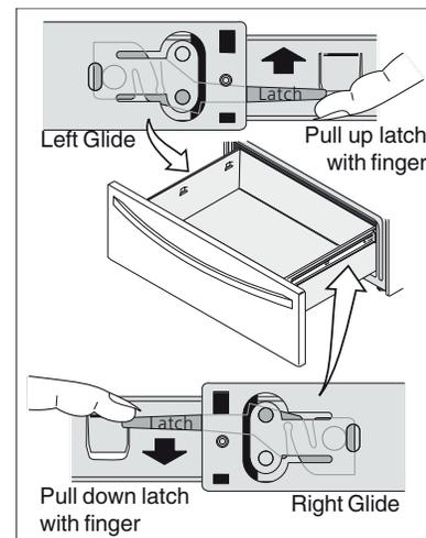
Figure 25: Parts of storage drawer
