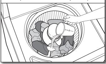
During the final rinse, wait until the washer has completed filling, then press the Start/Pause button to pause the washer. Lift the lid and add the measured recommended amount of liquid fabric softener. Do not use more than the recommended amount. Close the lid and press the Start/Pause button again to start the washer.
