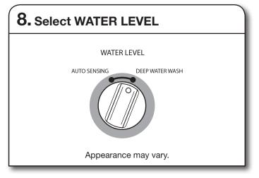
Set the Water Level knob to the Auto Sensing setting and the washer will automatically sense the appropriate water level for the load size and type. Select Extra Rinse for enhanced rinsing performance.
