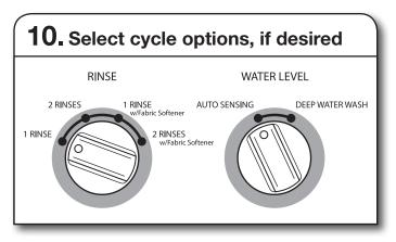
Select the number of rinses by turning the Rinse knob to the desired setting.
