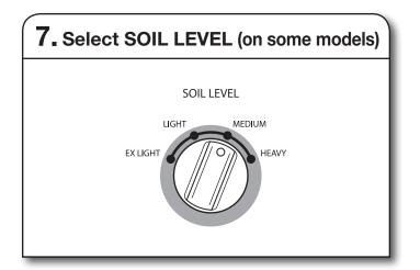
Once you select a cycle, select the soil level by turning the Soil Level knob to the desired setting.
