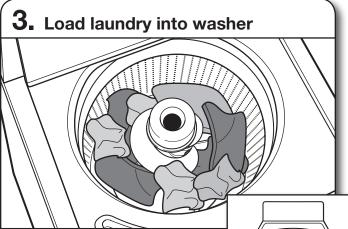
Load garments in loose heaps evenly around basket wall. For best results, do not pack the load tightly. Do not wrap large items such as sheets around the agitator; load them in loose piles around the sides of the basket. Try mixing different-sized items to reduce tangling.
