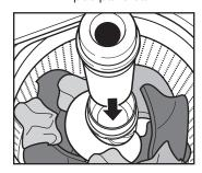
**Fabric Softener Dispenser** This convenient fabric softener dispenser connects to the agitator and saves you from manually adding fabric softener during the rinse cycle.
