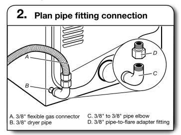
A combination of pipe fittings must be used to connect dryer to existing gas line. Recommended connection is shown. Your connection may be different, according to supply line type, size, and location.
