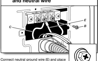
hooked end (hook facing right) of neutral wire (white or center wire) (C) of direct wire cable under center screw of terminal block (B). Squeeze hooked ends together and tighten screw.
