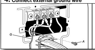
Connect a separate copper ground wire (G) from the external ground conductor screw (A) to an adequate ground. Finally, reinsert tab of terminal block cover into slot of dryer rear panel. Secure cover with hold-down screw. Now, go to "Venting Requirements."
