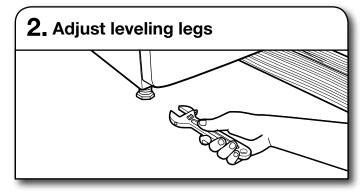
If dryer is not level, prop up using a wood block. Use wrench to adjust legs up or down, and check again for levelness.
