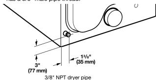
**NOTE:** For a garage installation, the gas pipe height must be an additional 18" (460 mm) from the floor.
