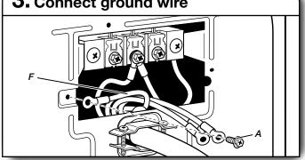
Connect ground wire (F) (green or bare) of power supply cord to external ground conductor screw (A). Tighten screw.
