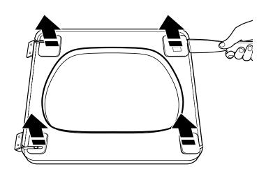
6. Using a #2 Phillips screwdriver, remove the remaining 4 screws from the hinges. Then remove hinges A and B and set both the screws and hinges aside.
