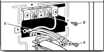
Remove center terminal block screw (B). Remove neutral ground wire (E) from external ground conductor screw (A). Reinstall ground conductor screw (A).
