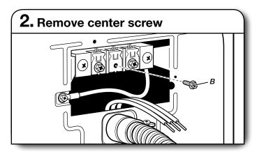
Remove center terminal block screw (B).
