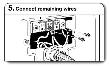
Place hooked ends of remaining direct wire cable wires under outer terminal block screws (hooks facing right). Squeeze hooked ends together and tighten screws. Finally, reinsert tab of terminal block cover into slot of dryer rear panel. Secure cover with hold-down screw. Now, go to "Venting Requirements."
