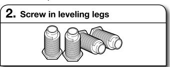
Using a wrench and tape measure, screw leveling legs into leg holes until bottom of foot is approximately 1" (25 mm) from bottom of dryer.
