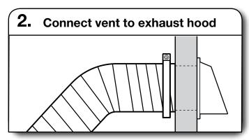
Vent must fit over the exhaust hood. Secure vent to exhaust hood with 4" (102 mm) clamp. Run vent to dryer location using straightest path possible. Avoid 90° turns. Use clamps to seal all joints. Do not use duct tape, screws, or other fastening devices that extend into interior of vent to secure vent, because they can catch lint.
