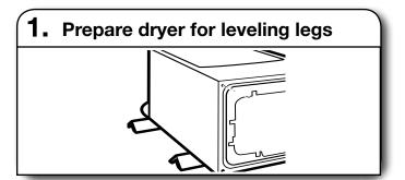
Firmly grasp dryer body (not console panel) and gently lay dryer down on back cardboard corner posts.
