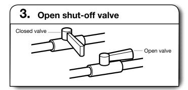
Open shut-off valve in supply line; valve is open when handle is parallel to gas pipe. Then, test all connections by brushing on an approved noncorrosive leak-detection solution. Bubbles will show a leak. Correct any leaks found.
