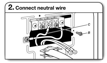
Connect neutral wire (white or center) (C) of power supply cord to center terminal block screw (B). Tighten screw.
