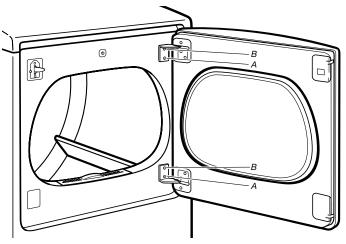
4. Remove the dryer door from the cabinet by lifting upward and out. Lay the door on a towel or a soft cloth you placed on a flat workspace.
