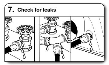
Check for leaks around "Y" connector, faucets, and hoses.
