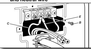
Connect neutral ground wire (E) and neutral wire (white) (C) of power supply cord under center terminal block screw (B). Tighten screw.
