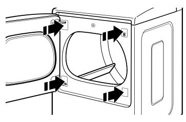
2. Hang the door on the unit by placing set pin in dryer cabinet hole and sliding door down. Using a Phillips screwdriver, install screws 1 and 3 and then screws 2 and 4. Tighten all hinge screws.
