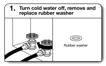
Turn cold water faucet off and remove washer inlet hose. Remove old rubber washer from inlet hose and replace with new rubber washer.
