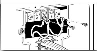
Connect remaining wires to outer terminal block screws Tighten screws.
