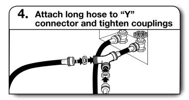
Attach dryer 5 ft (1.5 m) inlet hose ends to the "Y" connector. Attach washer cold inlet hose to other side of "Y" connector. Screw on coupling by hand until it is seated on connector. Using pliers, tighten the couplings an additional two-thirds turn.
