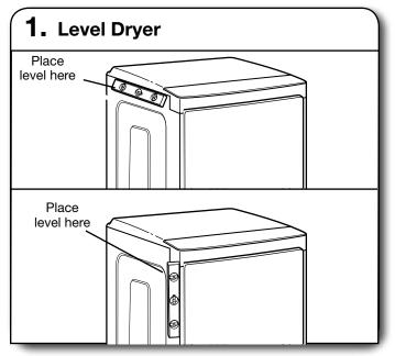
Check levelness of dryer from side to side. Repeat from front to back.
