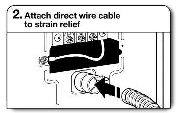
Put direct wire cable through the strain relief. The strain relief should have a tight fit with the dryer cabinet and be in a horizontal position. Tighten strain relief screw against the direct wire cable.
