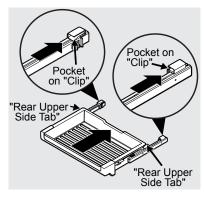
Apply pressure to drawer while supporting slide from below. Tab/clip passes through opening in drawer to locate. Ensure both sides are engaged.
