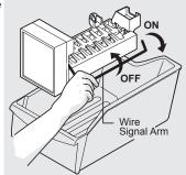
also turns off automatically when the ice container is full. If your model has an adjustable freezer shelf, place the shelf in the lower position, so that the wire signal arm will hit the ice when the container is full.
