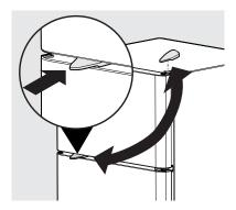
Tighten the top hinge screws and check door gasket for open seal condition (gap between gasket and cabinet flange).
