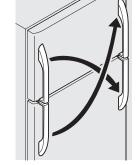
from freezer door and attach to the refrigerator door.
