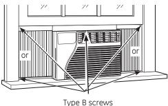
Extend the left and right accordion panels to the vertical window sashes and attach, through the holes in the panels, with 5 Type B screws.
