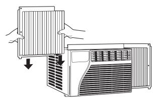
Slide the left and right accordion panels into the top and bottom mounting rails.
