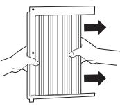
B Slide the free end of the accordion panel into the side panel rails. Slide the panel down. Be sure to leave enough space to slip the top and bottom of the frame into the rails on the cabinet
