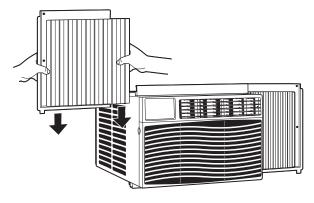
Slide the left and right accordion panels into the top and bottom mounting rails.
