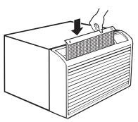
**NOTICE:** Do not operate the air conditioner without the filter in place. If a filter becomes torn or damaged it should be replaced immediately.
