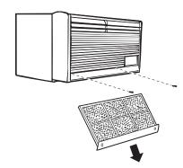
3. Pull the grille out from the bottom and lift up from the tabs on the top of the case.
