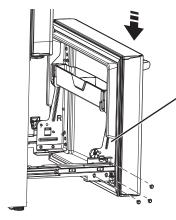
Align and insert tab on Freezer Door Bracket with slot on Freezer Slide Bracket.
