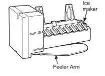
**NOTE:** In homes with lower-than-average water pressure, you may hear the ice maker cycle multiple times when making one batch of ice.
