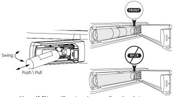
position. If filter will not swing easily, check to ensure filter is properly aligned and fully seated within the cartridge holder. Close the filter door.
