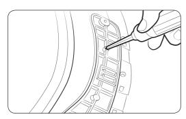
**10.** Insert the screw you just removed into the other screw hole on the back of the door hinge, and then tighten.
