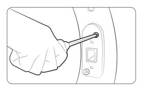
**12.** Push the lever holder into the cut out on the other side of the door opening. Insert screws, and then tighten as shown.
