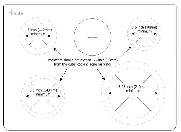
Fig. 1 - Induction cooking zones minimum pan size requirements
