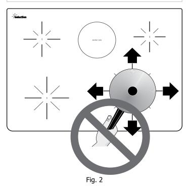
Sliding any type of cookware over the surface will scratch the cooktop over time. Scratches will make cleaning the ceramic cooktop difficult and degrade the appearance of the cooktop.
