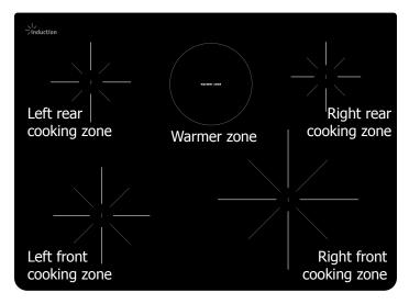
Induction cooking directly heats the pan; heating will only begin when cookware is properly placed on the cooking zones. For the best possible surface cooking results, it is recommended to only use high quality heavy gauge cookware on the induction cooking zones.
