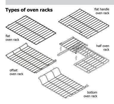
The **flat oven rack** or **flat handle oven rack** (some models) may be used for most cooking needs.
