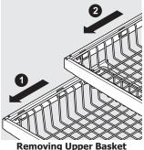
To reinstall upper basket, position basket onto the retainer clips making sure the front of the basket rests in the retainer clips on the stabilizer bar.
