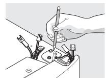
2 Disconnect the harness by grasping both sides of the connector firmly, depress the latch, and pull apart. Remove the two screws from the top hinge. Lift the door off of the bottom hinge and set it aside.
