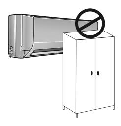
21. Do not place obstacles around air-inlets or inside of air-outlet. It may cause failure of appliance or accident.
