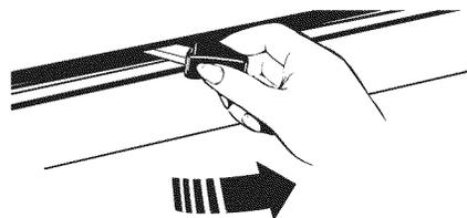
Soil on the front frame of the range and outside the gasket on the door will need to be cleaned by hand. Clean these areas with hot water, soap-filled steel-wool pads or cleansers such as Soft Scrub®. Rinse well with clean water and dry.
