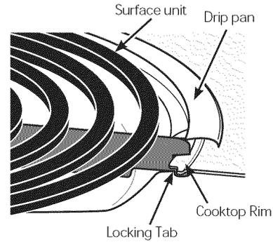
When properly seated, the locking tab should lock onto the cooktop rim through the notch in the drip pan.
