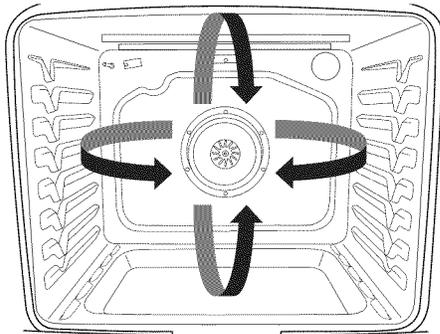
With convection cooking, most foods can be cooked at a temperature 25°F (15°C) lower than in a standard thermal oven, and cooking time can be shortened by up to 30%.
