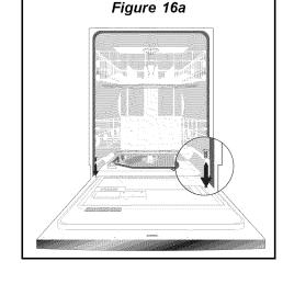
3. Place one hand on each side of door and pull down at top approximately 1/4".
