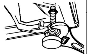
**16.** If washer is not level, repeat Step 11, and adjust the front legs up or down. Then repeat Steps 14 & 15.
