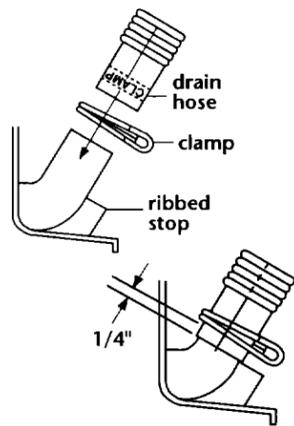
**6.** To prevent the drain hose from coming off or leaking, it must be installed per the following instructions.
