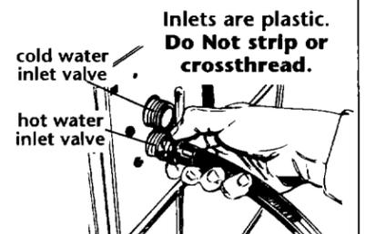
**5.** Attach one hose to the hot water (bottom) inlet valve first; then other hose to the cold water (top) inlet valve. Tighten couplings by hand. Then use pliers to make an additional two-thirds turn. **DO NOT OVERTIGHTEN;** this could cause damage to couplings.
