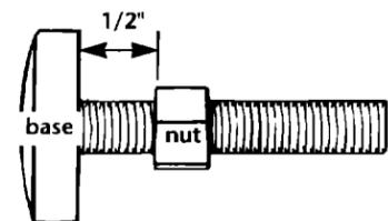
**12.** Screw nut down on legs to within 1/2 inch of base.
