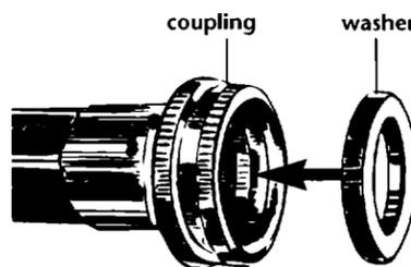
**4.** Insert a flat washer into each end of the inlet hoses. Check that washers are firmly seated in couplings.
