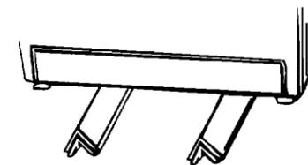
**11.** Stack two corner posts on top of each other. Tilt washer backwards and slide corner posts under washer 3 inches from each side of washer as shown.
