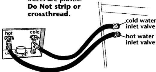
**10.** Attach bottom hose from the inlet marked "H" to the hot water faucet. Attach top hose from the inlet marked "C" to the cold water faucet. Tighten couplings to faucets. **DO NOT OVERTIGHTEN;** this could cause damage to couplings.
