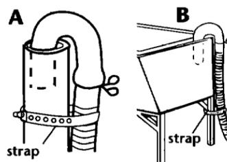
Put "hook" end of drain hose in laundry tub or standpipe. Tightly wrap the shipping strap around the drain hose and laundry tub or standpipe as shown in Figures A-B. Push plug into the nearest hole in the shipping strap.
