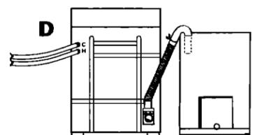
If a longer drain hose is needed, use a 21" or 54" drain hose and Connector Kit, Part No. 285442. If drain hose must be shortened, use Connector Kit Part No. 285442. These parts are available from your local dealer or authorized parts distributor.
