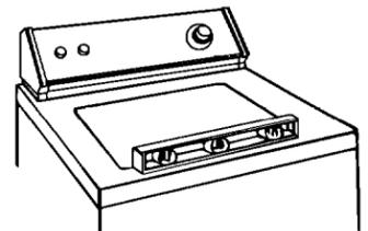
**15.** Tilt washer forward slightly so that back legs are about 1 inch off floor. Drop washer to floor. Check levelness of the washer by placing a carpenter's level on top of the washer, first side to side; then front to back.
