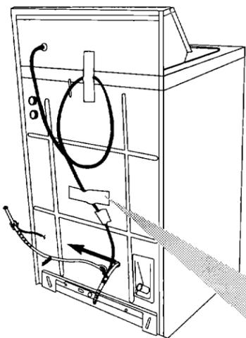
**SLIDE WASHER ONTO CARDBOARD OR HARDBOARD BEFORE MOVING ACROSS FLOOR.**
