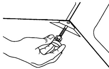
**13.** Insert legs into correct holes at each front corner of washer until nuts touch washer. **DO NOT** tighten nuts until Step 16.
