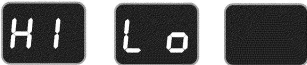
Figure 2: Range from Hi setting to Lo to OFF (blank display)
