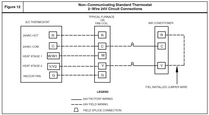
NOTE: Wiring must conform to NEC or local codes.
