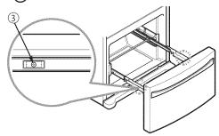
With the drawer pulled out to full extension, insert the lower basket (4) in the rail assembly.
