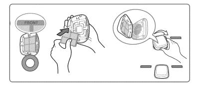
After changing the filter, push and hold the Air Filter button for three seconds to reset the filter sensor.
