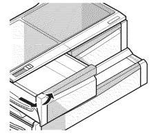
**3.** To install, slightly tilt up the front, insert the drawer into the frame and push it back into place.
