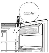
**4.** Press and hold the Freezer Temp button for three seconds while continuing to hold your phone to the speaker.
