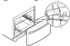
Lower the door into its final position and tighten the screws (3) located on both sides.
