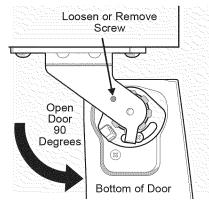
Loosen/Remove Screw (where applicable)
