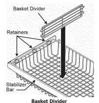
Lift up on the rear of the lower divider and pull out.
