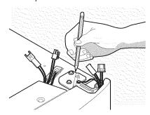
2 Disconnect the harness by grasping both sides of the connector firmly, depress the latch, and pull apart. Remove the two screws from the top hinge. Lift the door off of the bottom hinge and set it aside.
