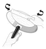
Figure 2: Check pan for flat bottom using ruler
