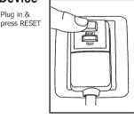
The power supply cord contains a current device that senses damage to the power cord. To test your power supply cord do the following:
