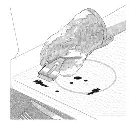
Figure 31: Using razor blade to remove burned on matter
