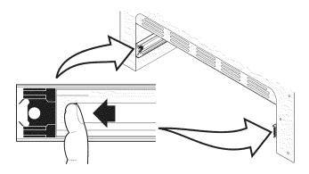
Figure 34: Bearing glide placement
