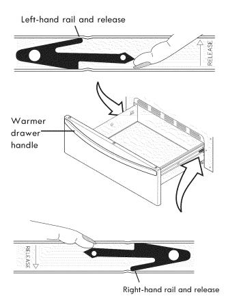
Figure 33: Removing the warmer drawer
