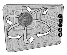
Figure 16: Air circulation in the convection function
