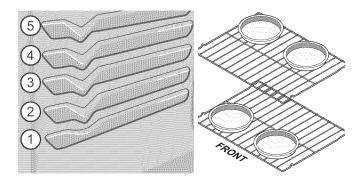
Figure 17: Convection rack positions and pan spacing
