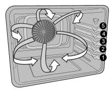
Figure 19: Air circulation in the convection roast
