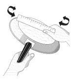
Figure 1: Check pan for flat bottom using ruler
