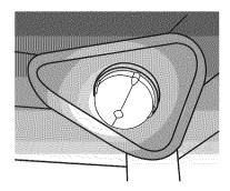
Figure 32: Replacing the oven light
