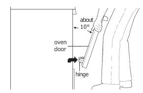
Figure 38: Holding door for removal
