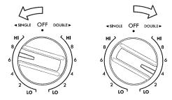
Figure 5: Dual radiant element control
