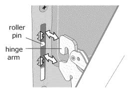
Figure 39: Location of hinge arm and roller pin
