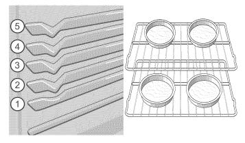
Figure 10: Rack positions and pan spacing recommendations
