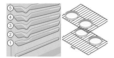
Figure 13: Convection rack positions and pan spacing
