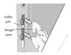
Figure 24: Location of hinge arm and roller pin
