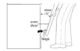
Figure 23: Holding door for removal
