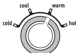
Once you select a cycle, select the desired wash temperature by turning the Temperature knob to the appropriate setting based on your load. All rinses are cold.
