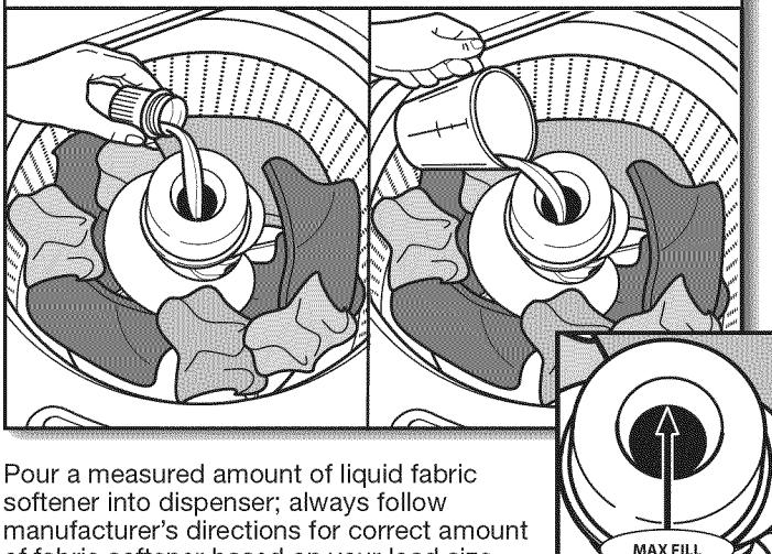
Pour a measured amount of liquid fabric softener into dispenser; always follow manufacturer's directions for correct amount of fabric softener based on your load size.
