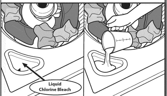
Do not overfill, dilute, or use more than 236 mL (1 cup). Do not use color-safe bleach or Oxi products in the same cycle with liquid chlorine bleach.
