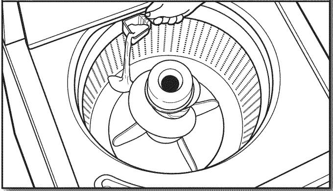
Add a measured amount of detergent into the bottom of the washer basket before adding clothes. If using an Oxi or color-safe bleach laundry boost product, add to the bottom of the washer basket, as well.
