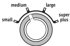
Select the Water Level setting most suitable for your load. Small will add a low amount of water for smaller loads and Super Plus will add the most amount of water for large or bulky loads. Items need to move freely.
