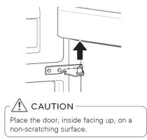
4 Remove the four screws **1**, the hinge pin insert **2** and the hinge pin brackets **3** from the bottom right side of the door.
