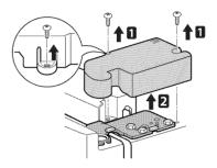
2 Using a 10mm or 13/32-inch socket wrench, remove the three bolts and lift off the top hinge. Set parts aside.
