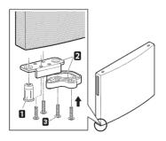
12 On the top part of the door, you will find a cap **1** and a pivot **2**. Remove them with a flat head screwdriver and install them on the opposite side ( the cap goes on the right and the pivot on the left).
