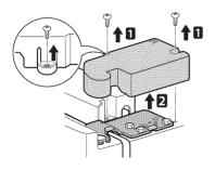
2 Remove the three bolts using a 10mm or 13/32-inch socket wrench and lift off the top hinge. Set parts aside.
