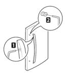
3 Carefully loosen the plug buttons with your fingers. The buttons can be unscrewed with the fingers by rotating them counter-clockwise and continuing until they loosen and fall out The buttons were installed without pressure, and for this reason, they can be unscrewed using your index finger, thumb or both. Install the plug buttons on the left side.
