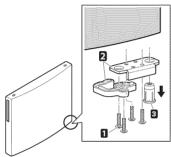
11 Reinstall the hinge pin insert **1**, the hinge pin brackets **2** and the screws **3** on the bottom left side of the door.
