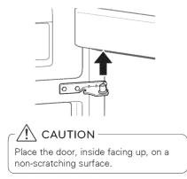
4 Remove the four screws (), the hinge pin insert (2) and the hinge pin brackets (3) from the bottom right side of the door.
