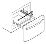
5 Grip both sides of the drawer and pull it up to remove it from the rails.
