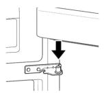
2 Line up the top hinge with the holes in the top of the refrigerator. Use the three bolts to replace the hinge. Tighten the bolts.
