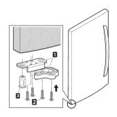
6 Use a ¼ inch hex socket wrench to loosen the hinge pin **1** and remove. Remove the two bolts **2**, the screw **3** and the hinge **4**.
