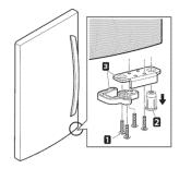
5 Reinstall the hinge pin brackets 1, screws
