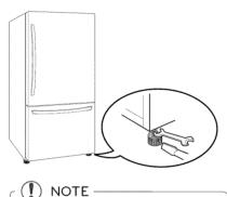
A flare nut wrench works best, but an open-end wrench will suffice. Do not over-tighten.
