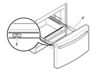
5 With the drawer pulled out to full extension, insert the lower basket in the rail assembly.
