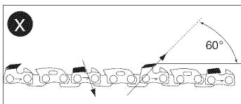
4. (Figure Y) Sharpen cutters (24) on one side of the chain first. File from the inside of each cutter to the outside. Then turn your saw around and repeat the processes (2,3,4) for cutters on the other side of the chain. Use a flat file to file the tops of the rakers (portion of chain link in front of the cutter) so that they are about .025 inch (.635 mm) below the tips of the cutters.
