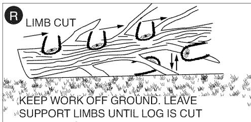
tension should be cut from the bottom up to avoid binding the chain saw. Trim limbs from opposite side keeping tree stem between
