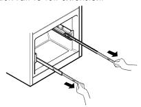
Grasp the drawer on each side and hook the drawer supports (1) into the rail tabs (2) located on both sides.
