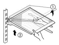
**To reinstall a shelf** — Tilt the front of the shelf up and guide the shelf hooks into the slots at a desired height.
