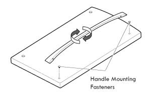
6. Install the handle by adjusting handle footprints to fit the mounting fasteners. Tighten the set screws with a 3/32 in. Allen wrench.
