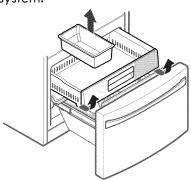
2. To replace, with the drawer pulled out to full extension, insert the top drawer in the rail assembly.
