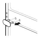
8. Remove the outer lower decorative screw from the flange on the frame between the freezer and refrigerator doors. (You will need this hole for the middle hinge bracket.)
