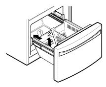
**NOTE:** Assemble the Durabase before assembling the middle drawer. The middle drawer needs clearance in order to properly seat its rollers. If the items are assembled improperly, the freezer door may not close.
