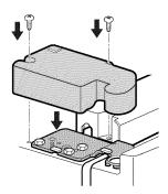
25. Replace the right hinge cap and insert the two screws.
