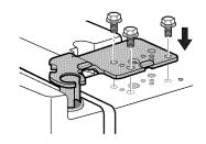
4 Replace the cover. Insert and tighten the cover screws (2).
