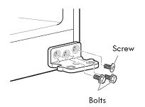
10. Remove the four screws (1), the hinge pin brackets (2) and the hinge pin insert from the bottom right side of the freezer door.
