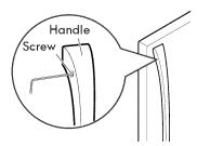
2. Loosen the handle mounting fasteners with a  $\frac{1}{4}$  in. Allen wrench.
