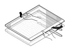
**To reinstall a shelf** — Slide the shelf into the guides until it stops.
