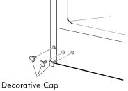
14. Using a 13/32 in. socket wrench with a 2 in. extension and a screwdriver, tighten the two bolts and a screw, and attach the bottom hinge on left side of the flange.
