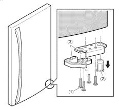
5. Reinstall the hinge pin brackets (1), screws (2) and hinge pin insert (3) on the bottom left side of the door.
