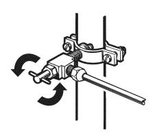
**CAUTION:** Check to see if leaks occur at the water line connections.
