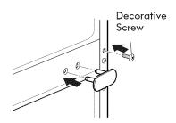
12. Loosen the two screws and remove the left hinge cap.
