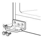
15. Attach the hinge pin using a  $\frac{1}{4}$  in. socket wrench.
