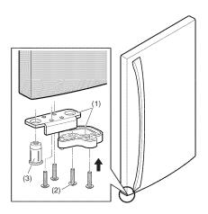
6. Use a 1/4 inch hex socket wrench to loosen and remove the hinge pin (1) from the middle hinge bracket. Use a10mm or 13/32 in. socket wrench to remove the two bolts (2). Remove the screw (3) and set the middle hinge bracket (4) and other parts aside.
