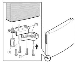
12. On the top part of the door, you will find a cap (1) and a pivot (2). Remove it with a flat head screwdriver and install it on the opposite side ( the cap stays on the right and the pivot on the left).
