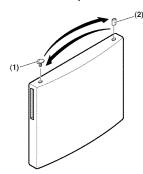
13. Remove the decorative caps on the bottom of the refrigerator housing. You will need these holes for the Bottom Hinge.
