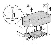
2. Using a 10mm or 13/32-inch socket wrench, remove the three bolts and lift off the top hinge. Set parts aside.
