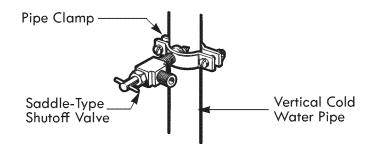
**NOTE:** Commonwealth of Massachusetts Plumbing Codes 248CMR shall be adhered to. Saddle valves are illegal and use is not permitted in Massachusetts. Consult with your licensed plumber.
