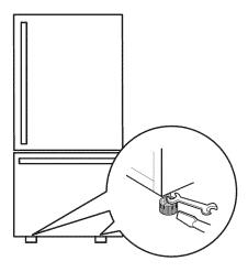
**NOTE:** Having someone push backward against the top of the refrigerator takes some weight off of the leveling legs. This makes it easier to adjust the legs.
